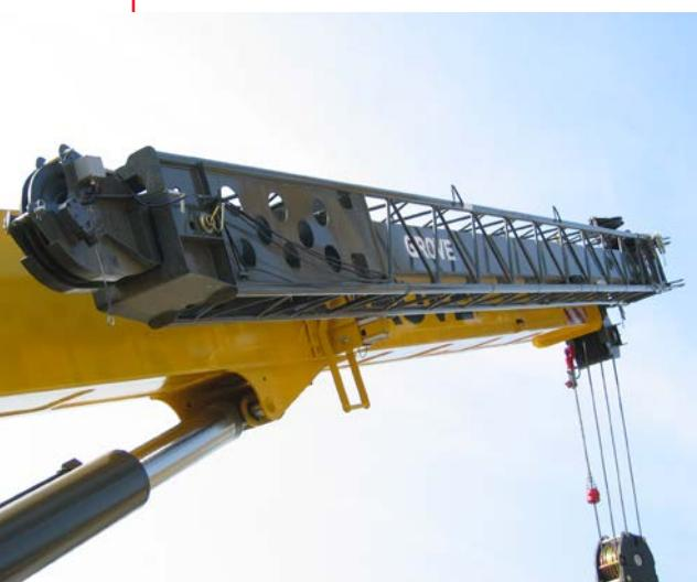
• **Extension:** An optional telescopic swingaway lattice extension easily stows on the side of the base boom for easy transport while providing on-board extension from 7,9 m - 13,7 m for a maximum tip height of 47 m.
